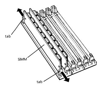
As you pull away the tabs, the SIMM falls to the left. When the SIMM is at an angle, release the tabs and carefully remove it from the socket.
